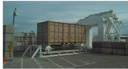
Gamma ( photofission ) and neutron ( differential die away ) induced fission systems
