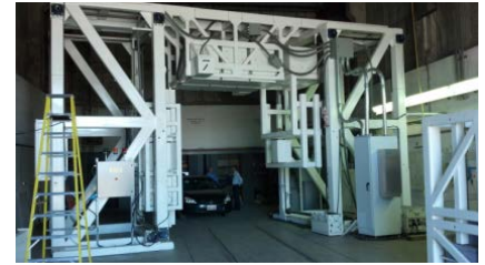
Gamma ( photofission ) and neutron ( differential die away ) induced fission systems
